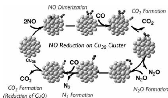
Scheme 3. New mechanism of NO reduction to N 2 via NO dimerization on Cu particle.
